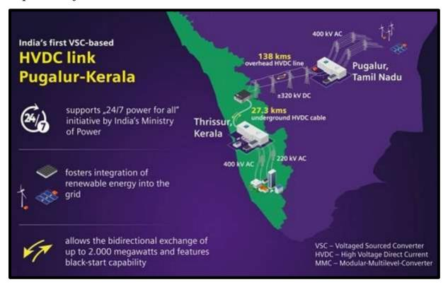
POWERGRID has totally commissioned India's 1st Voltage source converter (VSC) based mostly High Voltage direct current (HVDC) System.
